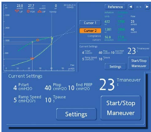
Figure 15: Settings for a recruitment maneuver with the P/V Tool using a fast pressure increase (ramp speed at 5 cmH 2 O/s), a pause of 10 s at high pressure, and higher PEEP after the recruitment maneuver
